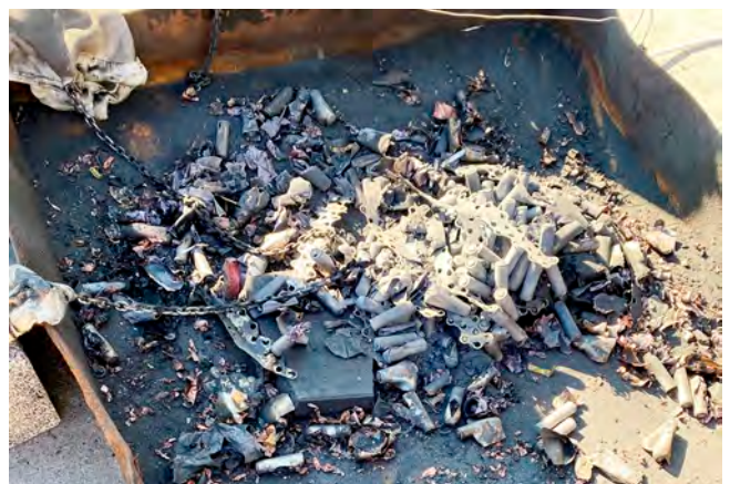
Photo 4: Phase 3 – The residues after completion of the fire test.
