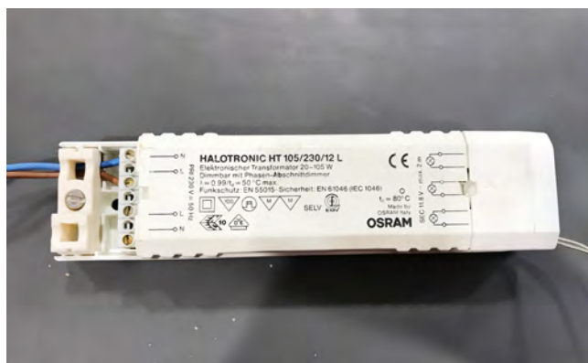
Photo 3: Electronic ballast unit (not suspected of containing PCBs).
