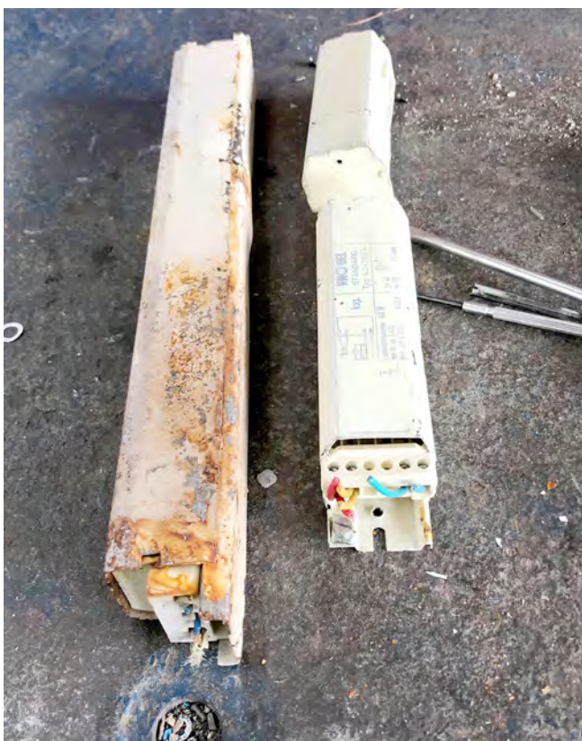
Photo 2: Two suspect ballast units found in a container with non-suspect ballast units during quality assurance. The electrical diagram on the right ballast unit points to the capacitor (capacitive part) with a symbol and the description "Kap".
